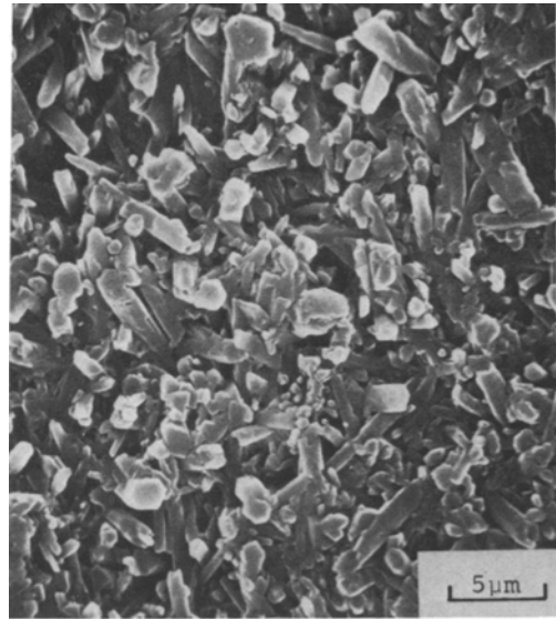
Figure 1 SEM of etched hot-pressed silicon nitride (NC-132) showing prismatic elongated grain structure. Apparent voids in the structure are the result of dissolution of silicates during etching in HF and pull-out of grains during preparation.
